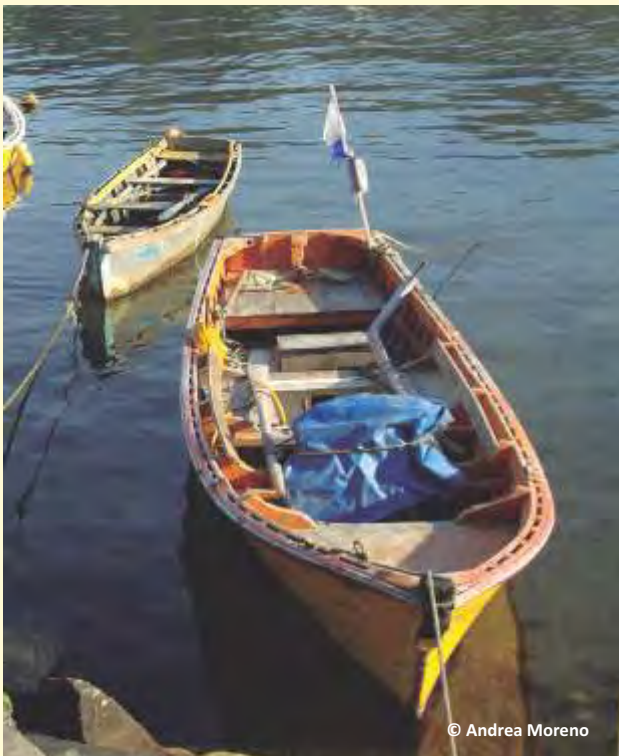
PHOTO 10. Undecked artisanal boats without engine.
