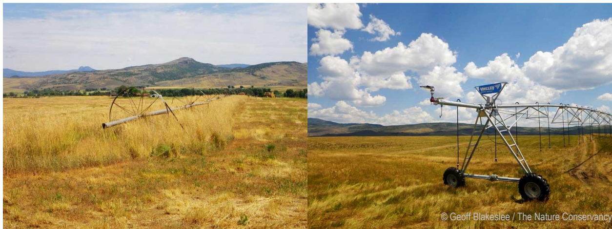
Figure 2. Side-roll wheel line irrigation used before project (left) and center pivot sprinkler irrigation used after project (right) at Carpenter Ranch Preserve (TNC, 2018).
