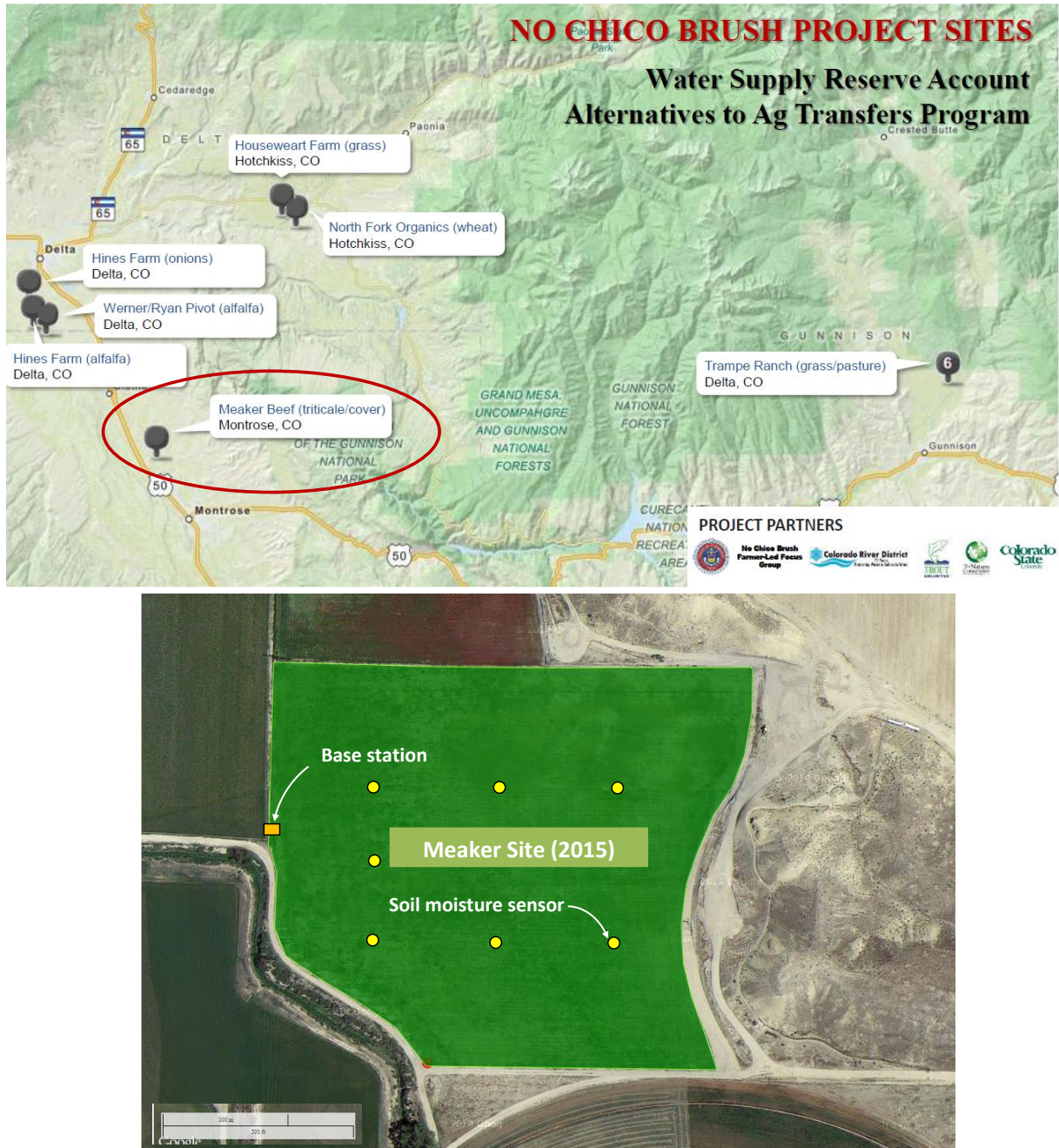
Figure 1. Map of the project location (top) and an aerial image of ~10 acres with improved irrigation technologies installed and monitored with flow meters and soil moisture sensors (bottom) (Cabot, 2015; Derwingson, 2016).
