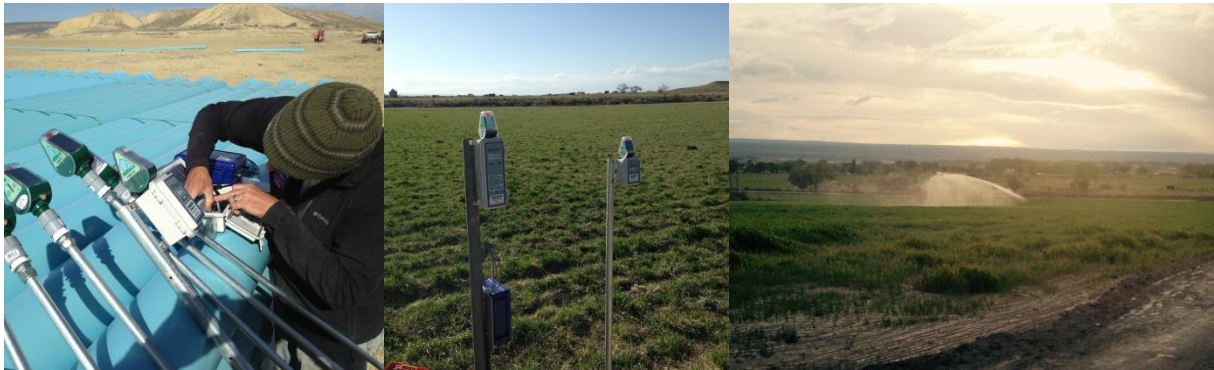
Figure 2. Dr. Cabot (CSU) prepares soil moisture sensors for installation (left); installed soil moisture sensors and communication relay units (middle); and big gun irrigation system in operation on Meaker Farm (right).
