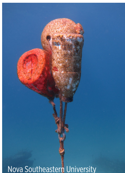
Figure 32. Example of plastic bottles or jerrycans for buoy. Flotation made of plastic may be used, but should be checked frequently, as any leak is a comprehensive failure.
