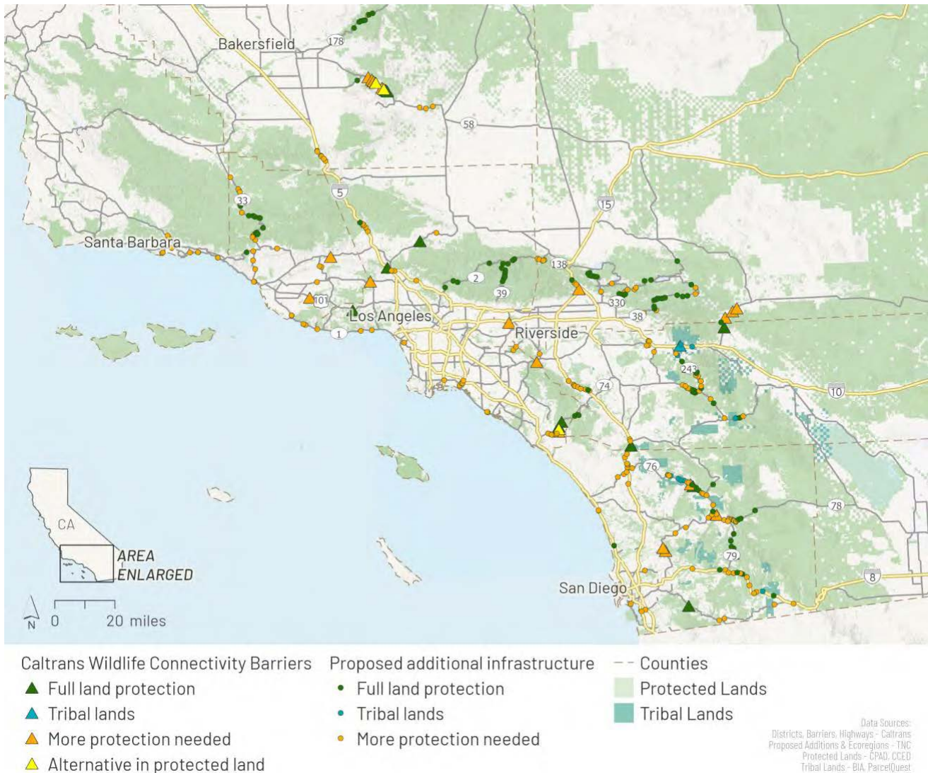
Figure 1. Map of infrastructure (bridges and culverts) in the South Coast and southern Sierra that can enhance wildlife connectivity and climate adaptation. Infrastructure is symbolized based on its surrounding land ownership.
