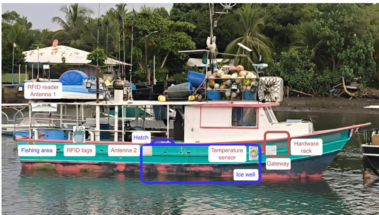
Figure 4: Physical installation locations of traceability equipment aboard the partner vessel.
