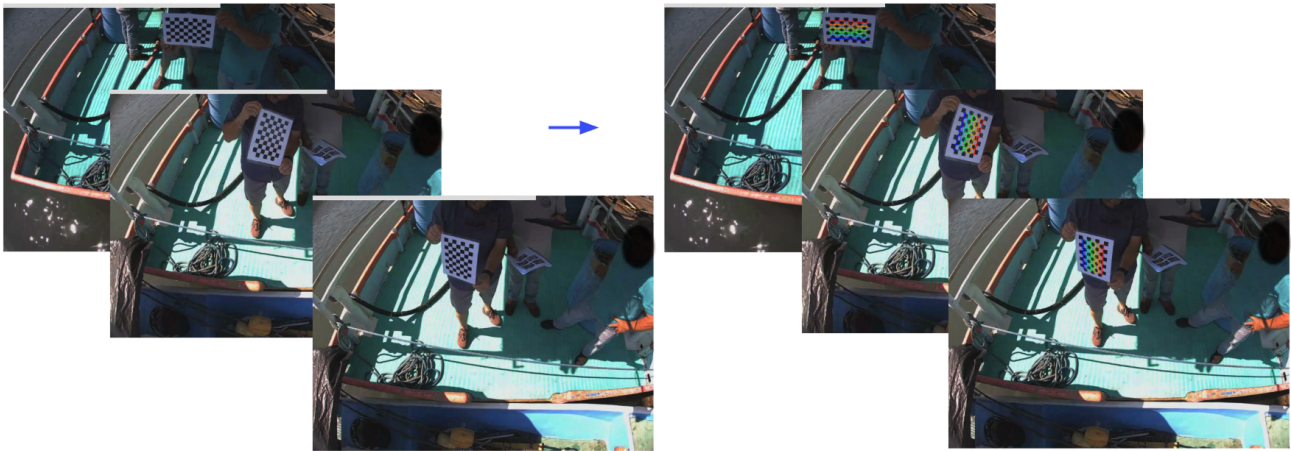
Figure 18. Sample chessboard calibration images used to correct camera distortion and prepare for size estimation.
