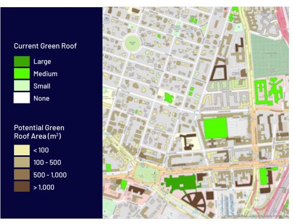
Figure 1: Map of potential green roof area for one portion of the district, showing existing green roofs on a few large buildings, primarily shopping centers, as well as potential future green roof area, with areas in dark brown indicating high potential for green roof construction.
