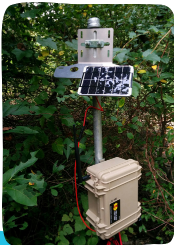
Below: The stream sensors are connected to a data logger device
