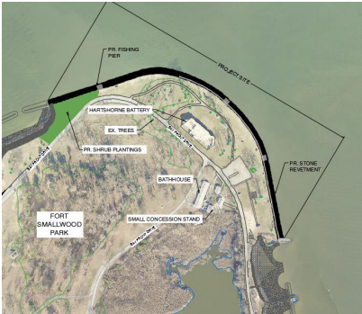
Stone revetment shoreline armoring on northern shore of park in 2021-2022
