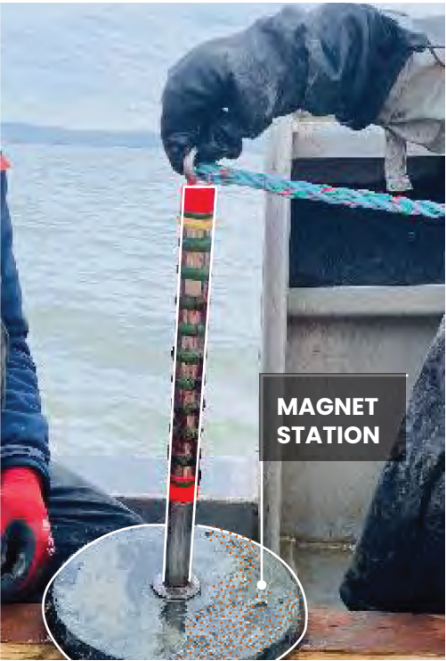
Nineteen magnet stations were installed one day after tracer deployment. Additional magnets were placed in tidal creeks to capture the trace.
