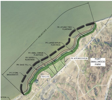
Shoreline armoring with stone breakwaters, sandy dredged material fill, and vegetation planting on northwestern shore of park in 2019
