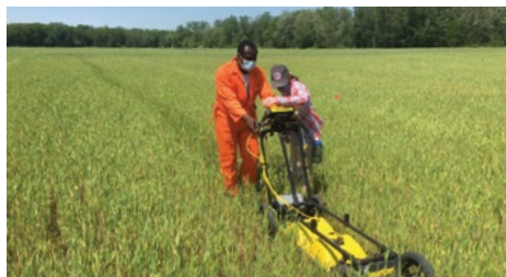
University of Toledo professor Kennedy Doro and student Anna Becker use ground-penetrating radar to detect hydrology infrastructure. © Alexis Sakas/TNC
