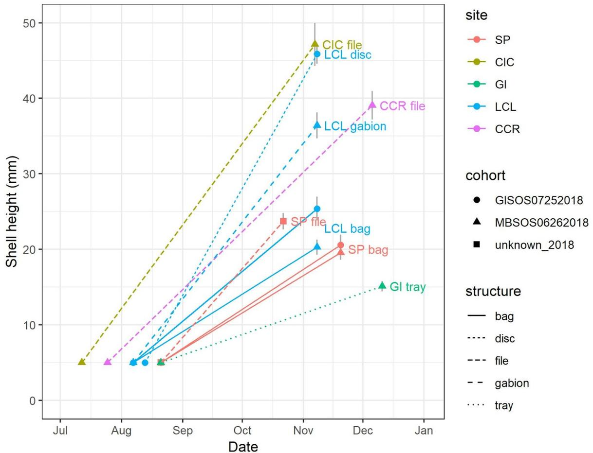
**Figure 9.** Oyster shell height over time for oysters installed in 2018 at Canarsie Community Reef (CCR), Coney Island Creek (CIC), Governors Island EcoDock (GI), Lemon Creek Lagoon (LCL), and the Sunset Park (SP) Community Reef and bagged shell reef. Error bars indicate 95% confidence intervals. “unknown\_2018” cohort is a mix of GISOS07252018 and MBSOS06262018.
