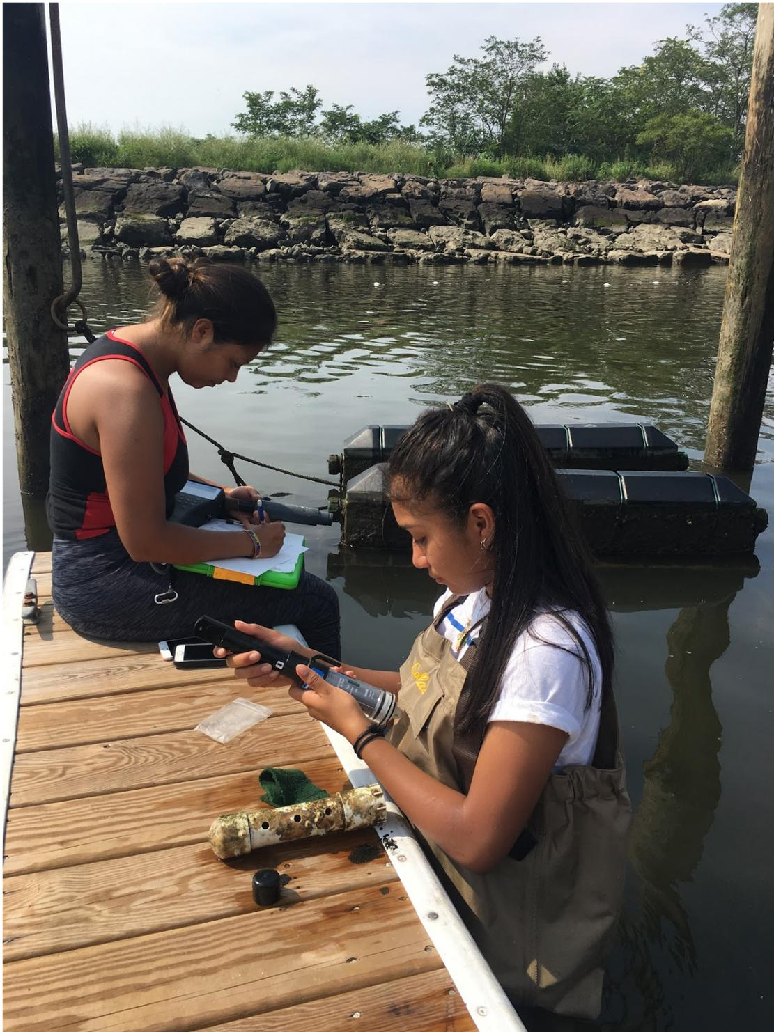
**Figure 32.** TNC Marine Science Technician Tatiana Castro-Gallego and BOP Summer Intern Lisette Mejia monitor water quality with HORIBA water quality meters and maintain HOBBO logger equipment.
