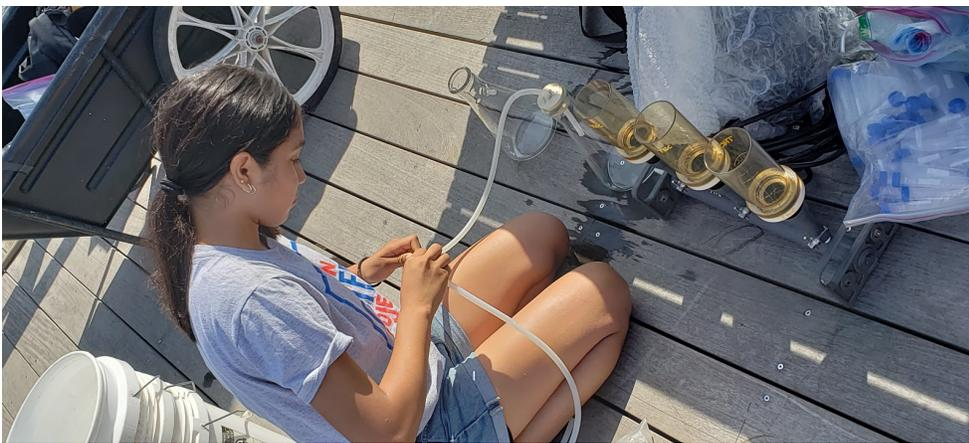
**Figure 40.** BOP Summer Research Intern Lisette Mejia sets up the vacuum filtration system to filter water samples for chlorophyll analysis.
