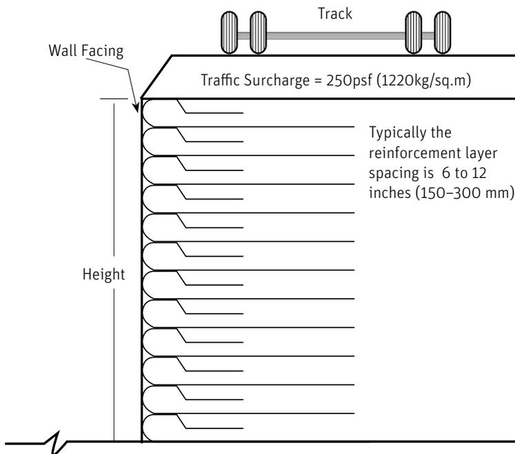
**Figure 10. Geotextile Wall Supporting Roadway Prism**
