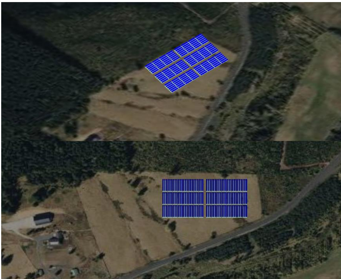
Figure 18. Centralia 43's agrivoltaic design using fixed tilt arrays with 12.3 ft spacing between rows (top). Agrivoltaic design using single axis tracking arrays with 9.8 ft spacing between rows (bottom). Rows of crops are underlaid.
