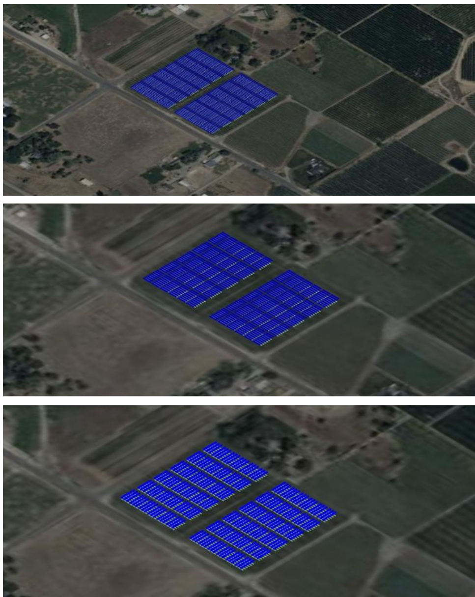
Figure 25. Stonemetz Orchards - agrivoltaic array designs using single-axis tracking arrays at low density (top), single axis tracking arrays at high density (middle), and fixed tilt at low density (bottom). Rows of trellised apple trees follow the orientation and spacing in the orchard.
