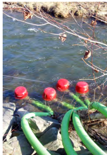
Each well uses an average of 4.4 million gallons of water. This water is transported from local stream and groundwater sources to the well pad with trucks or pipelines. © Susquehanna River Basin Commission
