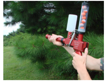
A burn crew member demonstrates the PyroShot launcher. © Drone Amplified
