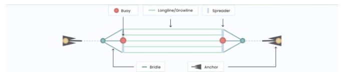
Figure 6. Five-line array illustration by Greenwave.
