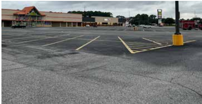
Excess impervious areas cause hotter temperatures and increased runoff. This parking lot could be retrofitted to add more trees, bioswales, and pervious surfaces that let water seep into the ground.
