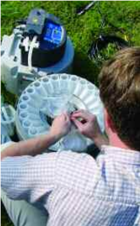
The durable and waterproof monitoring stations collect up to 24 samples, which are noted by date, time and corresponding water level.
