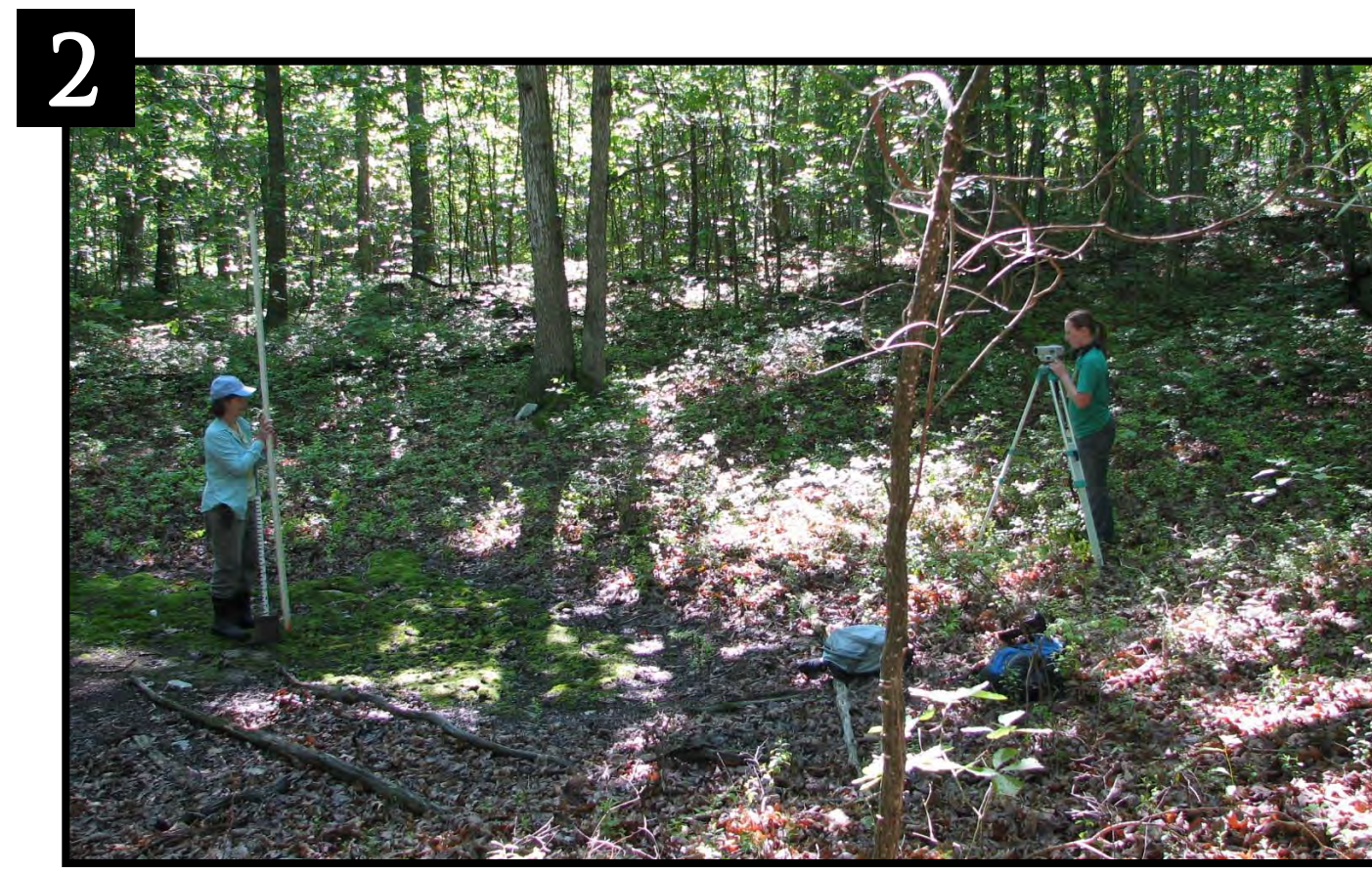
2 The size of the liner and maximum depth of each pool was determined by measuring the basin dimensions using a construction level and survey rod.
